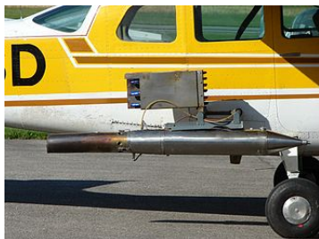
Cessna 210 equipped with a silver iodide generator for cloud seeding
