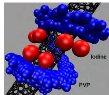
Schematic of povidone-iodine complex wrapping a single wall carbon nanotube (black).<sup>[18]</sup>
