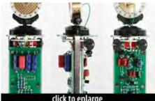
click to enlarge The circuit of the ST55 is nearly identical to the circuit of the GT55. The same circuit shows up (albeit without switched features) in the <u>M-Audio Luna</u>.
