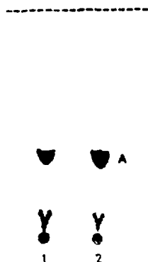
Fig. 1. Autoradiograph of TLC plate of aqueous extracts produced from Phaeodactylum tricorneratum (1) and Chlorella ovalis (2). The exposed area (dark) shows the presence of radioactive arseno organic compounds. The main compound is marked A. More detail is shown on the original film. Analytical condition: Cellulose substrate (1 mm); developing solvent, chloroform/methanol/ammonia, 2/2/1 (system 1).
