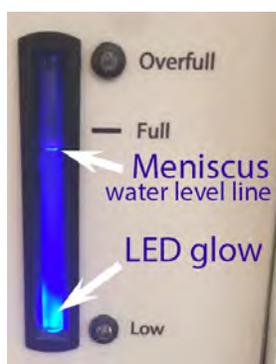
We added the blue LED and a floating ball to make it easier to see the liquid level, but the ball can (usually temporarily) get stuck.
