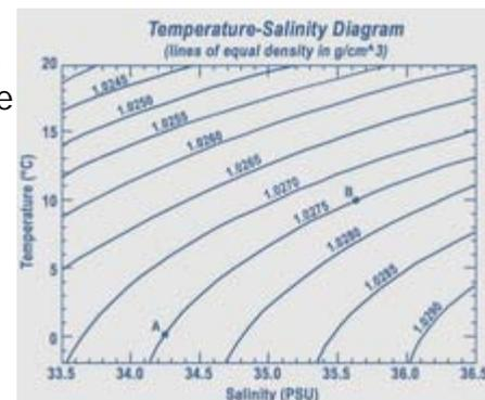
Temperature-salinity diagram of changes in density of water
