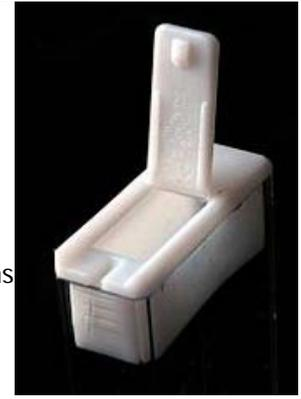
[Polypropylene](#) lid of a [Tic Tac](#) box, with a [living hinge](#) and the resin identification code, 5, under its flap
