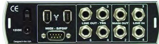
**12VDC Power Adaptor Input.** This is where you plug the provided power supply into the FIREBOX. Please check the power supply to ensure that it is the correct voltage and plug type for your country. Note that you can also power your FIREBOX with a six-pin FireWire port from your computer instead of using the external power supply.
