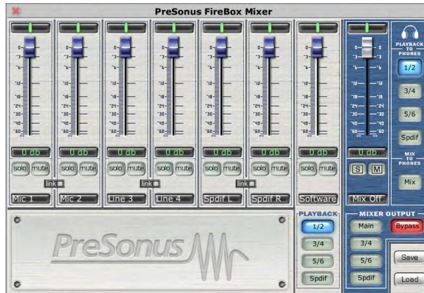
**NOTE:** The default settings (pictured above) for the FIREBOX mixer has all faders set to 0dB and all pans set to center, with the Software Playback set to channels 1/2, the Mixer Output set to Bypass, and the Playback to Phones set to channels 1/2.
