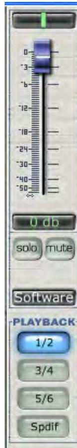
**Input (software playback channel)** – This is the audio return from your audio software. The same functions are available as the other inputs including PAN (balance between left and right channels), LEVEL, SOLO and MUTE. This is a stereo channel. This channel picks up the audio stream that is sent from your software and enables you to mix it with the direct input of your FIREBOX.
