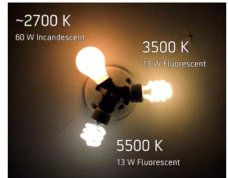
Color temperature comparison of common electric lamps<sup>[9]</sup>
