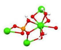
Portion of the lattice of dicalcium phosphate dihydrate, highlighting the 8-coordinated Ca<sup>2+</sup> center and the location the protons on three ligands (green = calcium, red = oxygen, orange = phosphorus, white = hydrogen)
